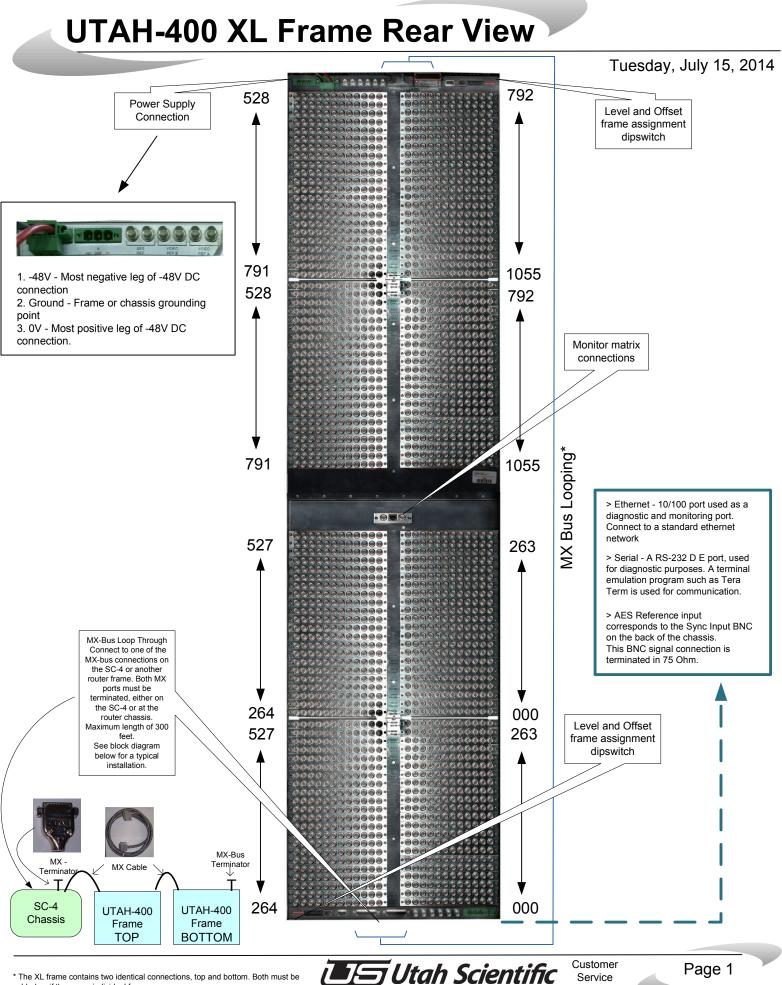
The XL frame contains two identical connections, top and bottom. Both must be cabled as if they were individual frames.
